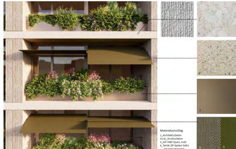
Fig. 4.12 left: Façade structure and materiality of the residential slab (source: hochform architects)
